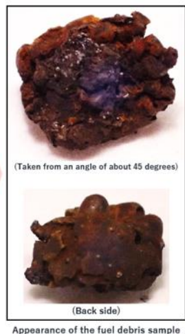
(Trial retrieval of fuel debris completed on Nov. 7, 2024)
