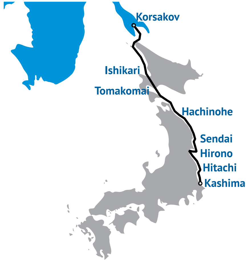
Figure 1. Proposed Subsea Pipeline Route*
